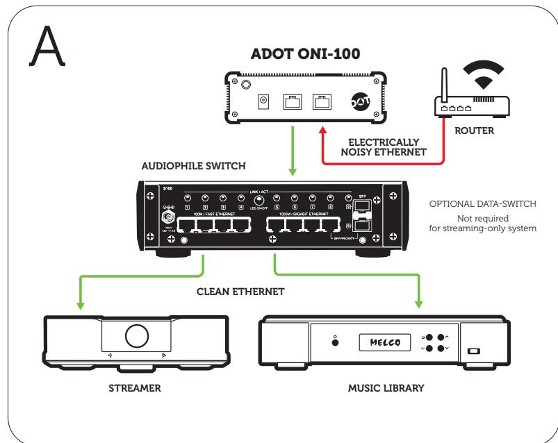
**1. There is no setting up required,** simply connect the *INPUT* socket to the residential network or router, and the *OUTPUT* socket to your HiFi System, or the Audio Data switch if that is used in the Hi-Fi system.
