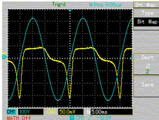
The display now shows the effect of applying the asymmetric load. The current in the transformer is now far from symmetric. It should also be noted that the small imbalance in current is not visible in the voltage (blue) trace, showing that very small offsets to the supply waveform have large effects on the operation of the transformer. If we were only monitoring the source voltage these effects would not be apparent.
