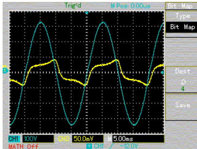
We have now introduced the filter unit inline with the sample transformer and the symmetric current trace is restored to its previous shape, showing that the filter has isolated the sample transformer from the effect of the asymmetric load on the mains supply.
