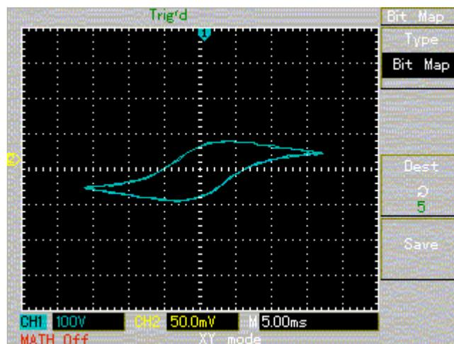
This now shows the classic hysteresis curve for the core of the transformer, rotated slightly by the inductive nature of the isolation transformer supplying the test setup.
