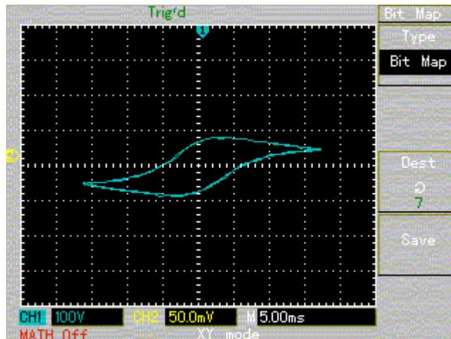
Again, the XY plot now shows the losses in the core are now back to just the hysteresis ones, and that the addition of the filter prevents the offset load from affecting the sample transformer.
