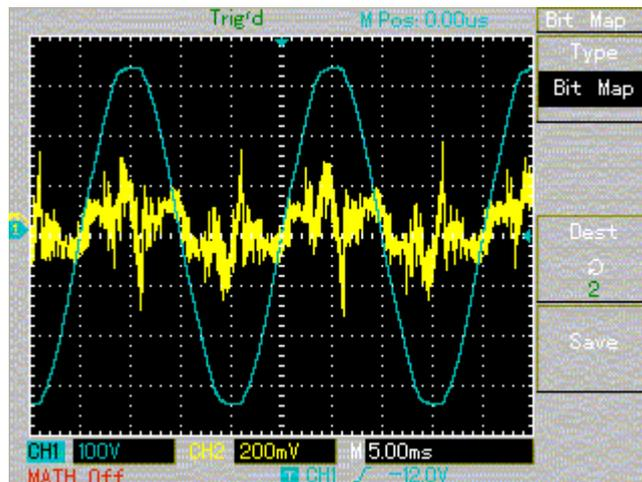
Once again, inserting the corrective filter into the supply, with the heat gun running, restores the display showing that the effect of the uneven load is removed, and the display is restored to its off load state.
