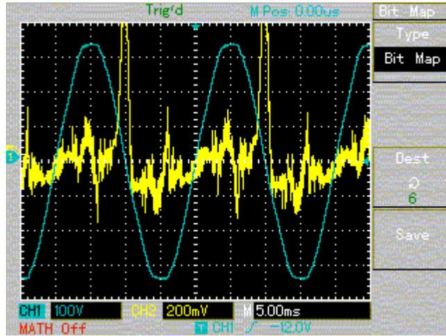
Turning on the heat gun instantly removed any doubt as to if the effect of the asymmetric load would be measurable. The same peaks are seen as were found in the controlled tests.
