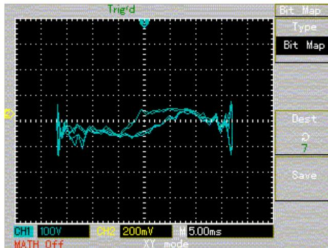
Again the corresponding Voltage/Current phase display. The hysteresis curve is still visible, but is now obscured by the high noise level, and the distortion of the sine wave at its peaks.
