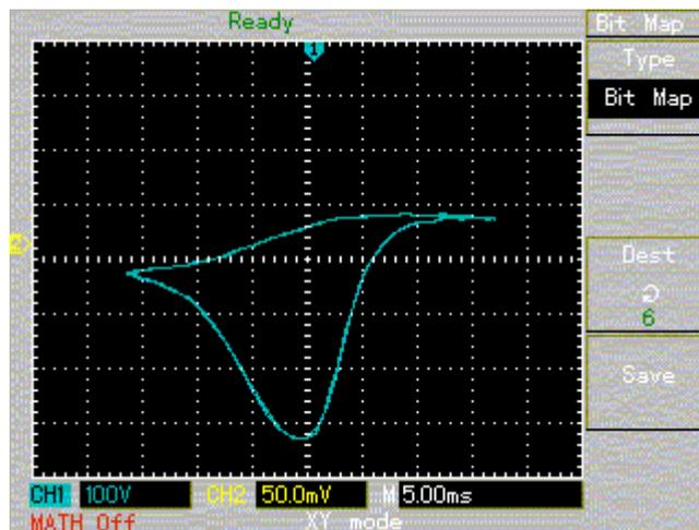
The corresponding XY display of the system shows how the losses in the transformer have increased (the area inside the curve is directly proportional to the energy loss in the transformer)
