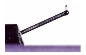
The boron cantilever and the diamond with "Super Linear Contact" cut - fitted "nude" - are as cleanly manufactured as the entire pickup.
