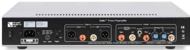
ABOVE: Separate MM and MC inputs will support two tonearms simultaneously while the MC input also includes continuously variable loading (1ohm-1kohm). RIAA eq'd outputs are offered on RCAs and balanced XLRs
