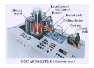
Because of its characteristics of single crystal, unidirectional, free of impurity, flexible fatigue-resistance, corrosive-resistance, low electric resistance, none-crystal boundaries, rapid transmissibility, perfect in structure, and easy to process, all make it an ideal material for making rapid transmission lines. From inner hook up wires to interconnect cables, they can be widely applied to Hi-Tech products such as Hi-Fi stereo system, high resolution TV.
